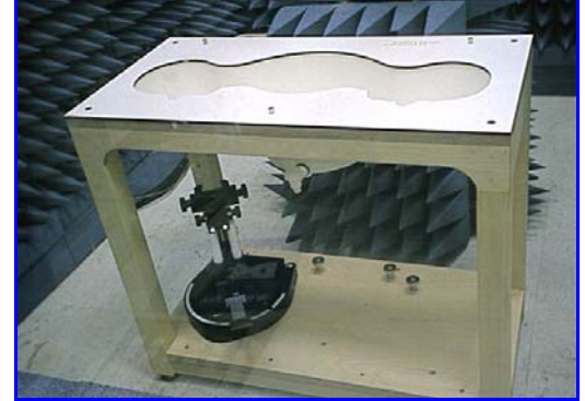
Figure 10. SAM Twin Phantom
