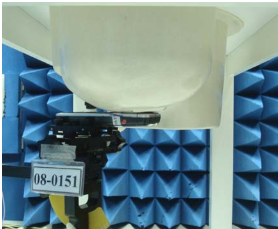
Figure 16. Left Head SAR Test Setup (Cheek)
