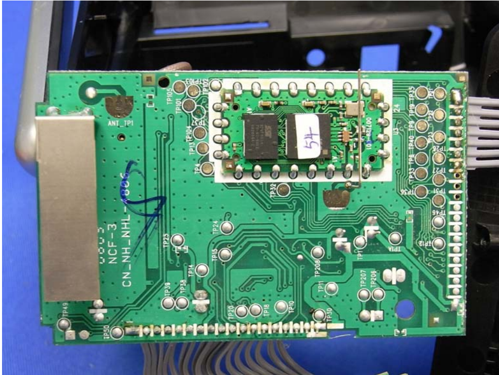
DECT RF Module PCB solder side and Bluetooth Module PCB comp side (View 1)
