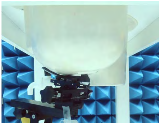
Figure 15. Left Head SAR Test Setup (Cheek)
