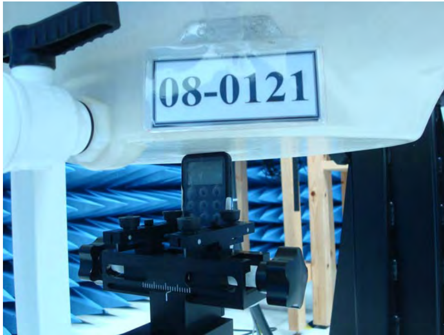
Figure 19. Body SAR Test Setup _ Tip to Phantom (0mm space)
