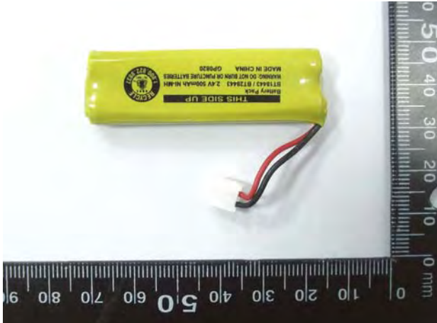
Figure 2. Battery (Ni-MH 2.4V , 500mAh)
