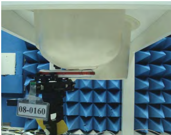
Figure 16. Left Head SAR Test Setup (Cheek)
