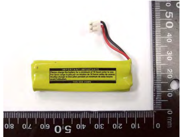
Figure 2. Battery (Ni-MH 2.4V , 500mAh)
