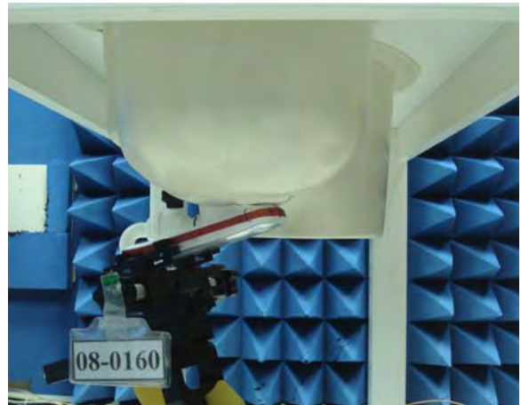
Figure 17. Left Head SAR Test Setup (Tilted)
