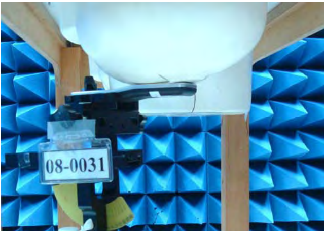
Figure 17. Left Head SAR Test Setup (Cheek)
