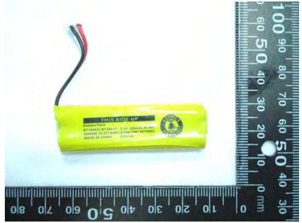
Figure 2. Battery (Ni-MH 2.4V , 500mAh)
