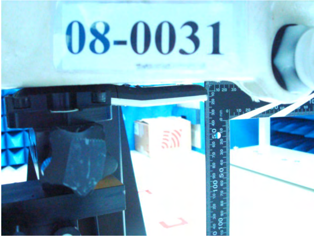
Figure 19.Body SAR Test Setup_ (Flat Section)
