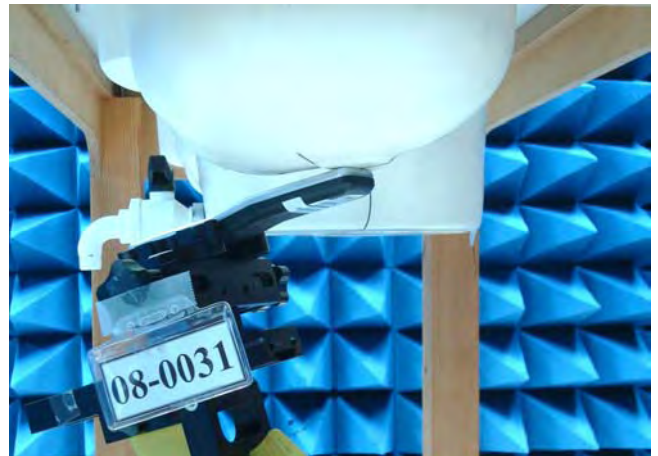
Figure 18. Left Head SAR Test Setup (Tilted)
