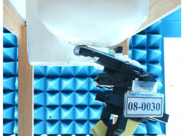
Figure 16.Right Head SAR Test Setup (Tilted)
