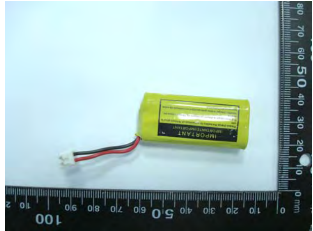
Figure 2. Battery (Ni-MH 2.4V , 600mAh)
