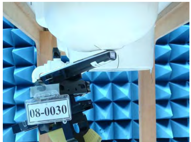
Figure 18.Left Head SAR Test Setup (Tilted)
