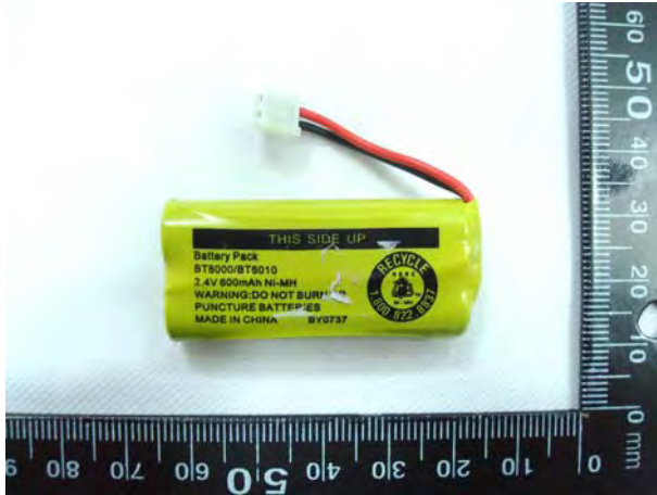
Figure 2. Battery (Ni-MH 2.4V , 600mAh)
