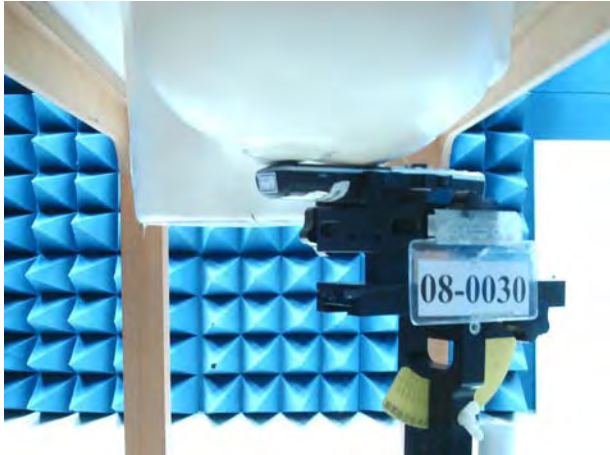
Figure 15.Right Head SAR Test Setup (Cheek)
