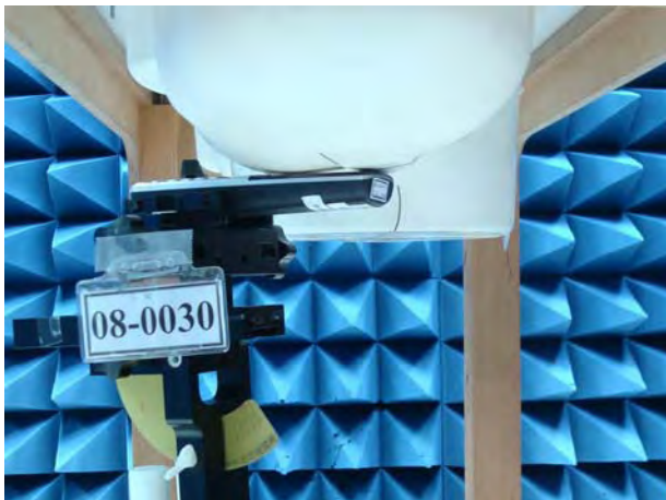
Figure 17.Left Head SAR Test Setup (Cheek)
