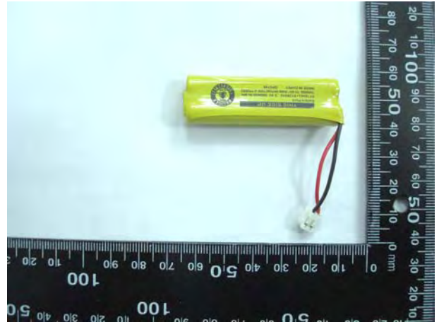
Figure 2. Battery (Ni-MH 2.4V , 500mAh)
