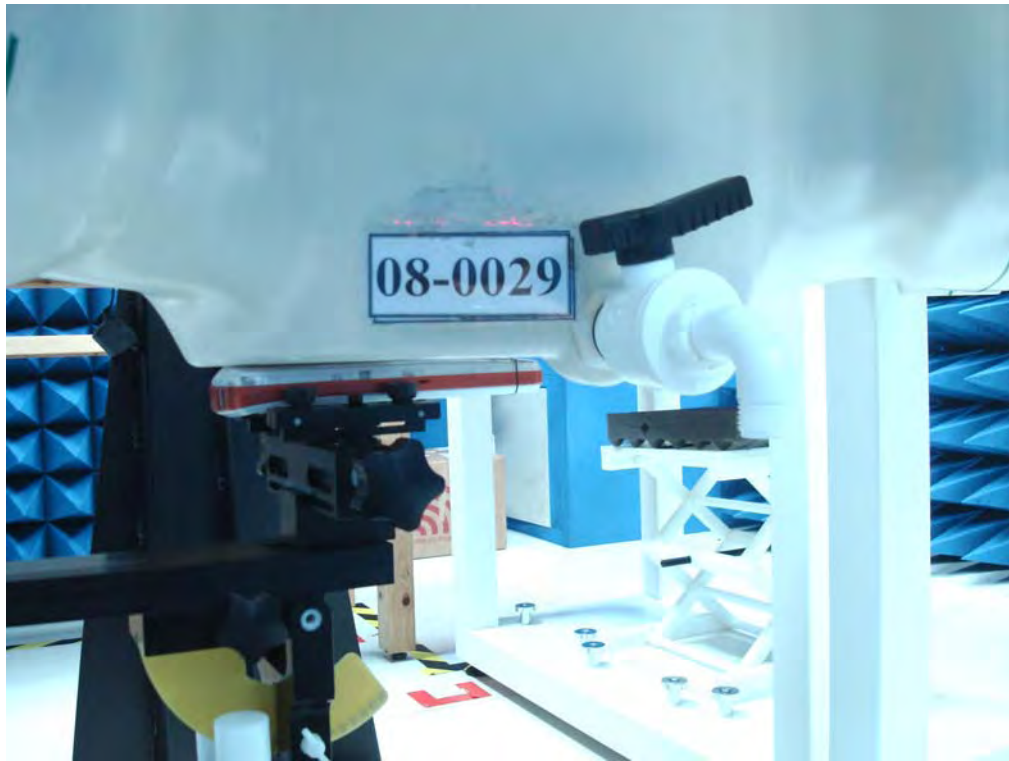
Figure 18. Body SAR Test Setup_ (Flat Section)
