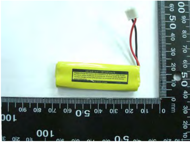
Figure 2. Battery (Ni-MH 2.4V , 500mAh)
