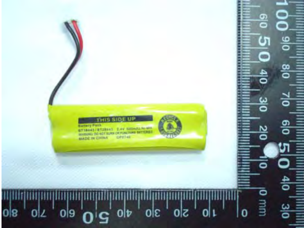
Figure 2. Battery (Ni-MH 2.4V , 500mAh)
