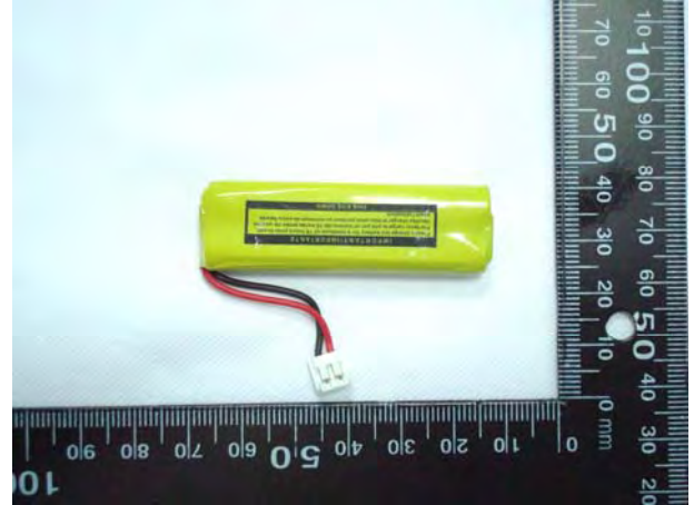
Figure 2. Battery (Ni-MH 2.4V , 500mAh)
