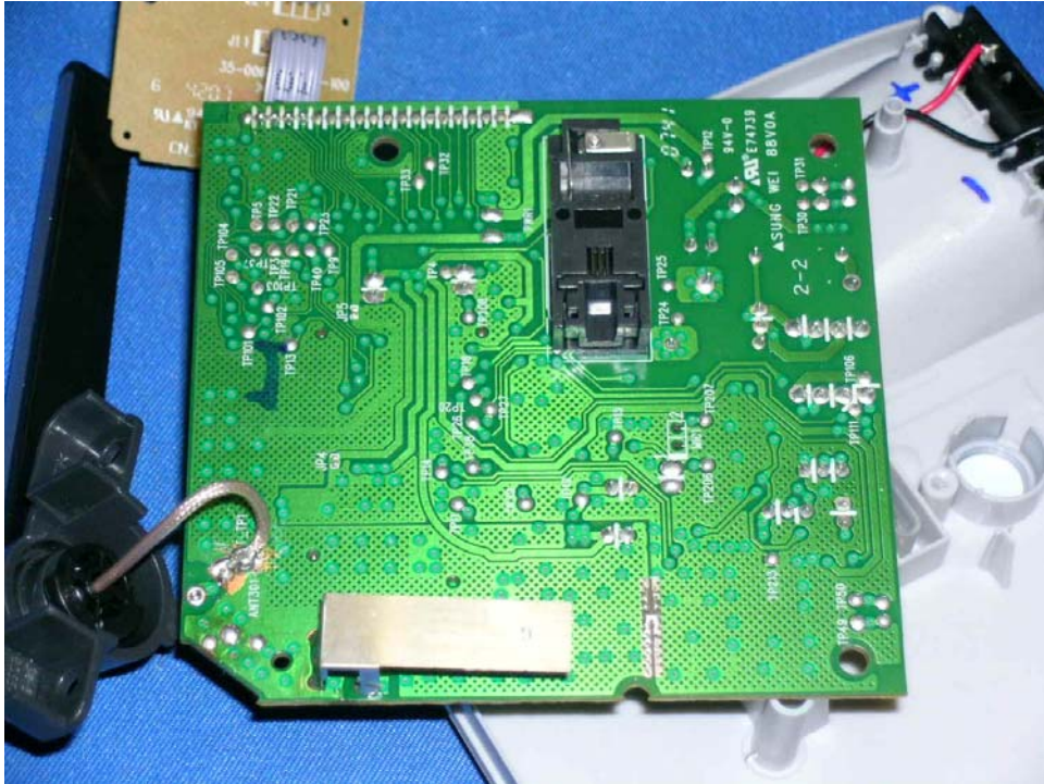
Base Unit Main PCB solder side
