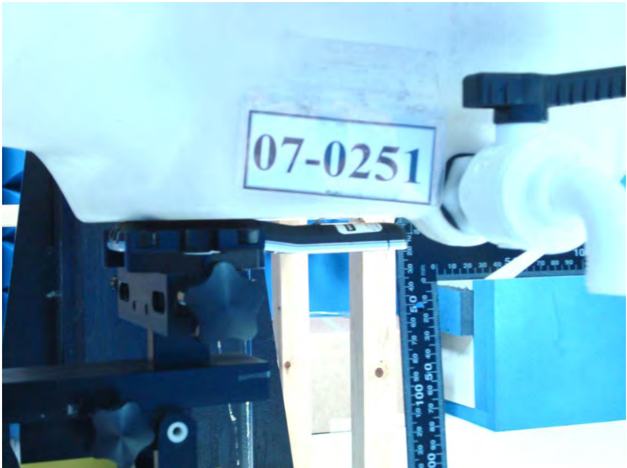
Figure 18. Body SAR Test Setup (Flat Section)
