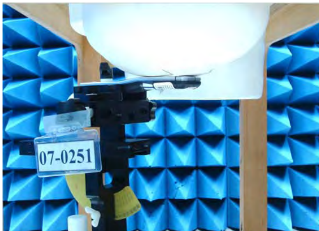
Figure 16. Left Head SAR Test Setup (Cheek)
