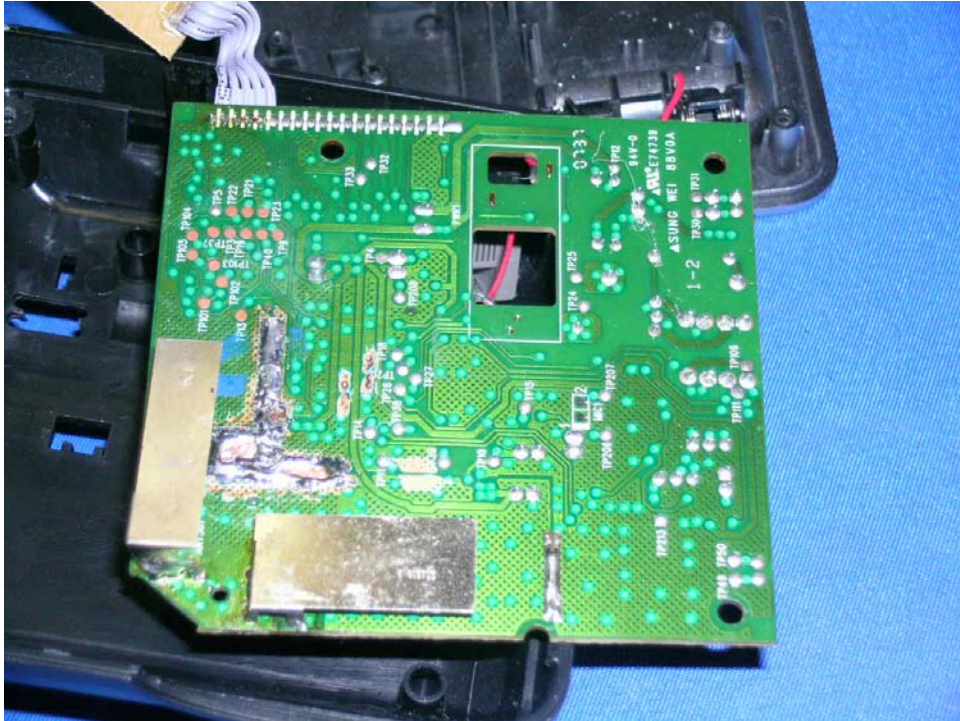
Base Unit Main PCB solder side
