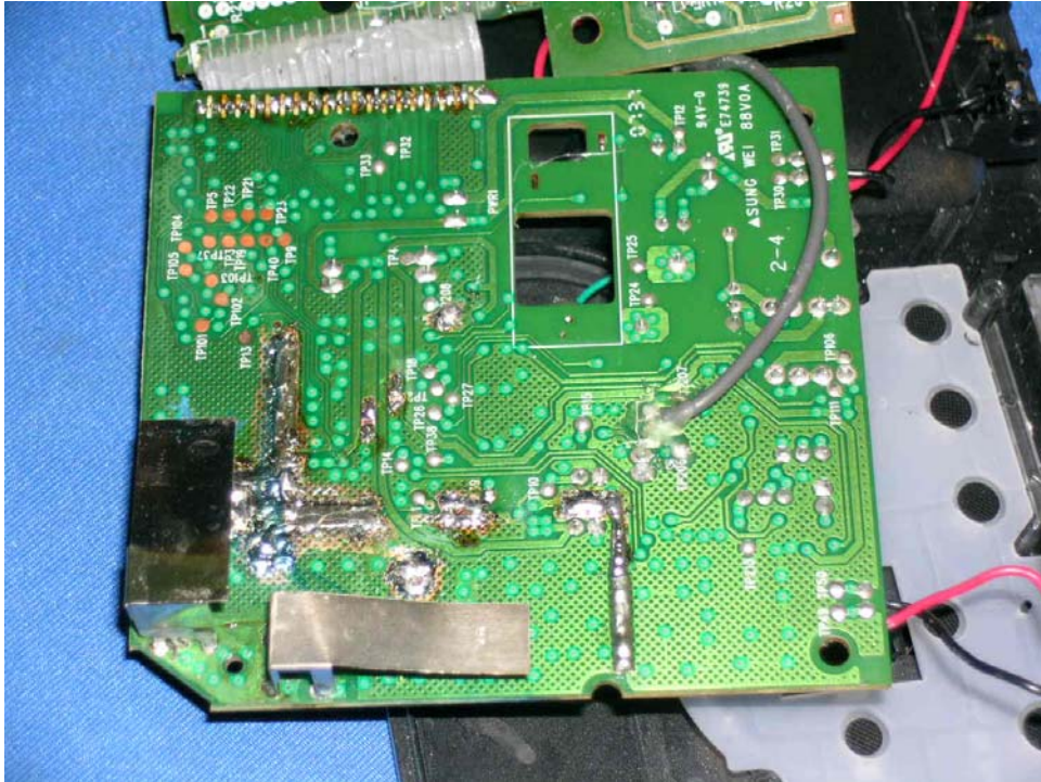
Base Unit Main PCB solder side
