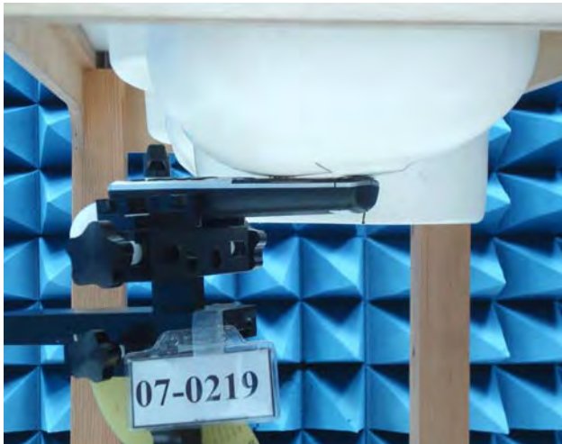
Figure 16. Left Head SAR Test Setup (Cheek)
