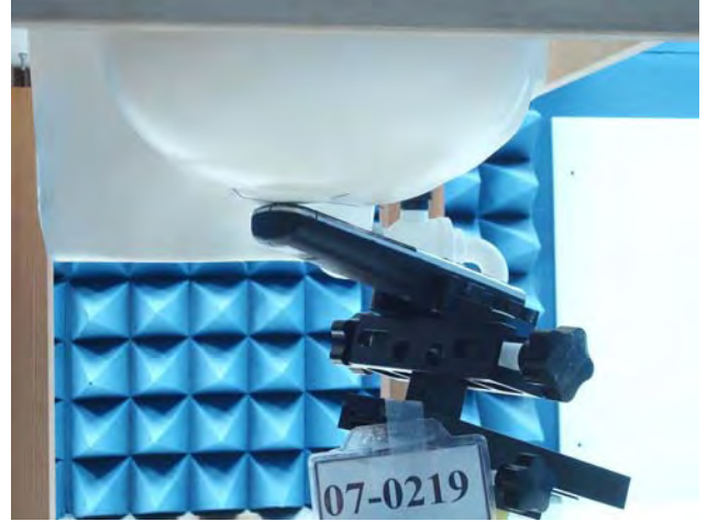
Figure 15. Right Head SAR Test Setup (Tilted)
