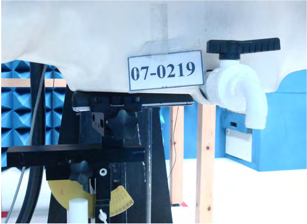
Figure 18. Body SAR Test Setup_ (Flat Section)
