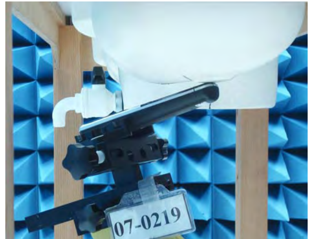
Figure 17. Left Head SAR Test Setup (Tilted)
