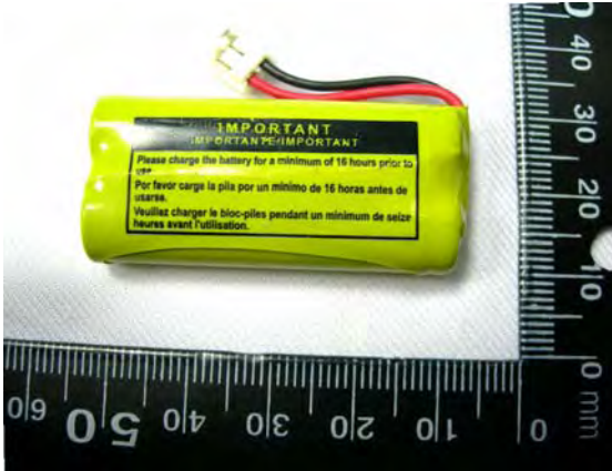
Figure 2. Battery (Ni-MH 2.4V , 600mAh)
