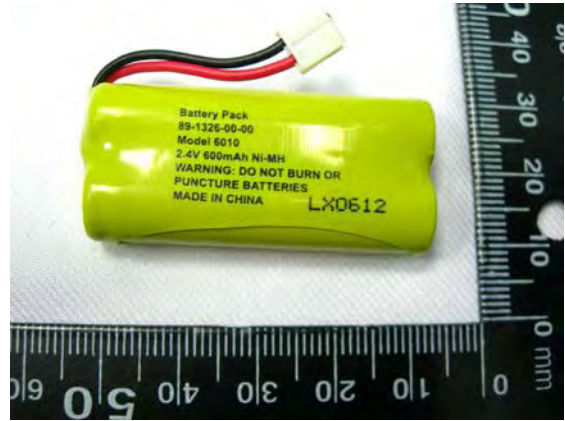
Figure 2. Battery (Ni-MH 2.4V , 600mAh)
