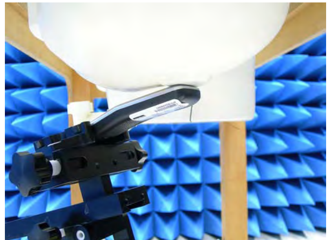
Figure 17. Left Head SAR Test Setup (Tilted)
