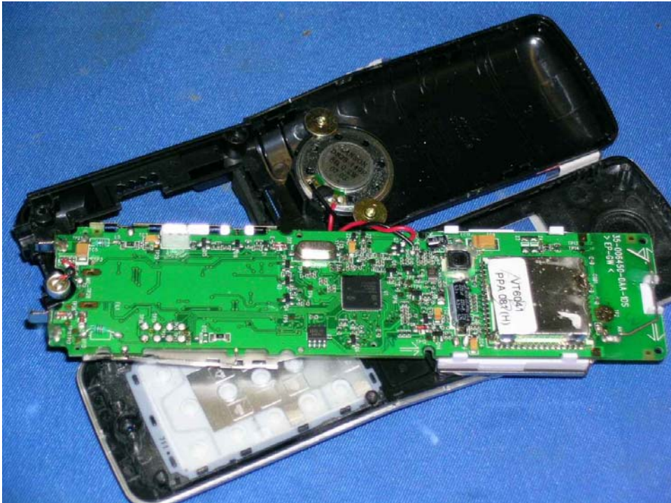
Handset Main PCB comp side
