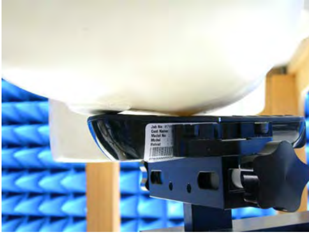
Figure 15. Right Head SAR Test Setup (Cheek)
