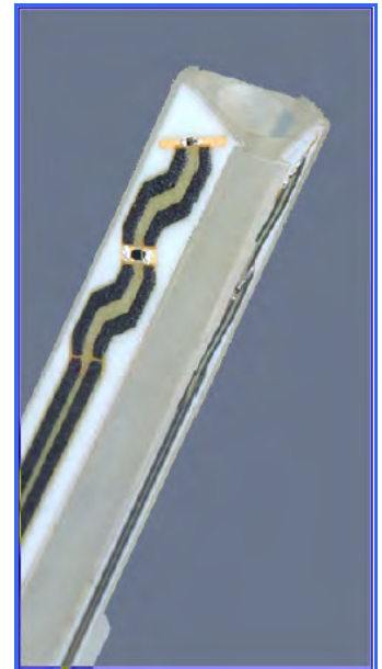
Figure 8. EX3DV3 E-field Probe
