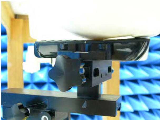
Figure 17. Left Head SAR Test Setup (Cheek)
