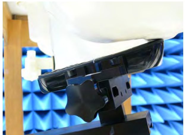
Figure 18. Left Head SAR Test Setup (Tilted)
