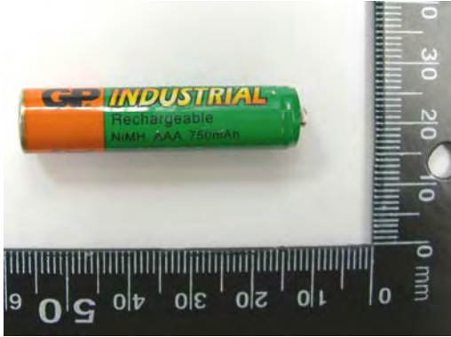
Figure 2. Battery (Ni-MH 1.2V × 2 , 750mAh)
