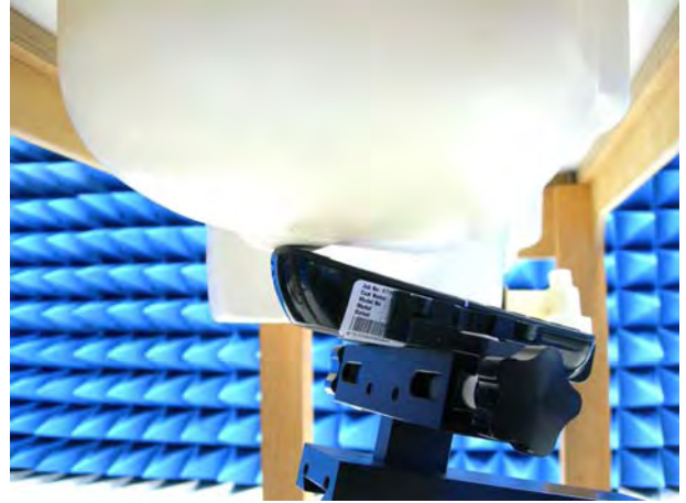
Figure 16. Right Head SAR Test Setup (Tilted)
