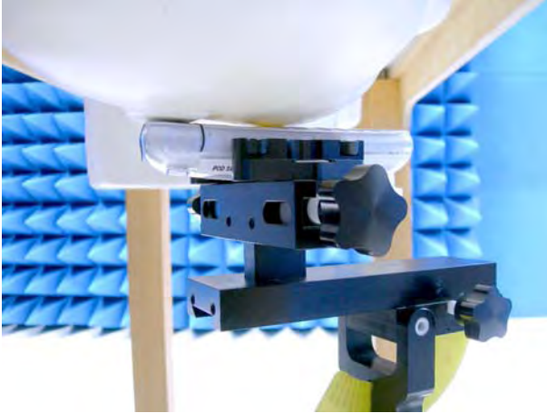
Figure 14. Right Head SAR Test Setup (Cheek)
