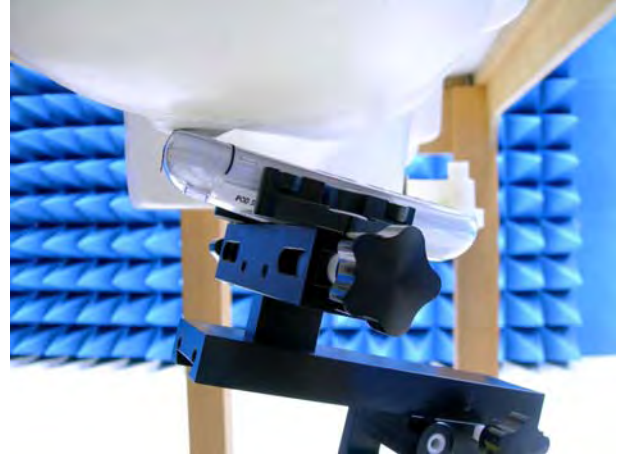
Figure 15. Right Head SAR Test Setup (Tilted)
