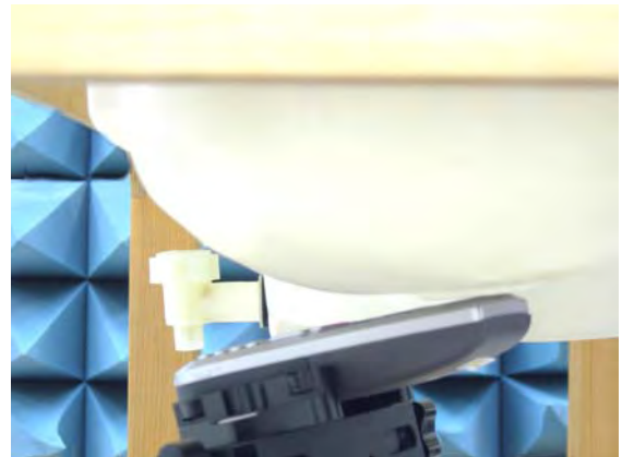
Figure 16. Left Head SAR Test Setup (Tilted)
