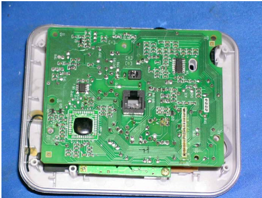
Base Unit Main PCB solder side
