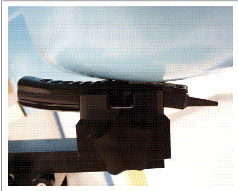
Setup Photo: Left Head Cheek Configuration
