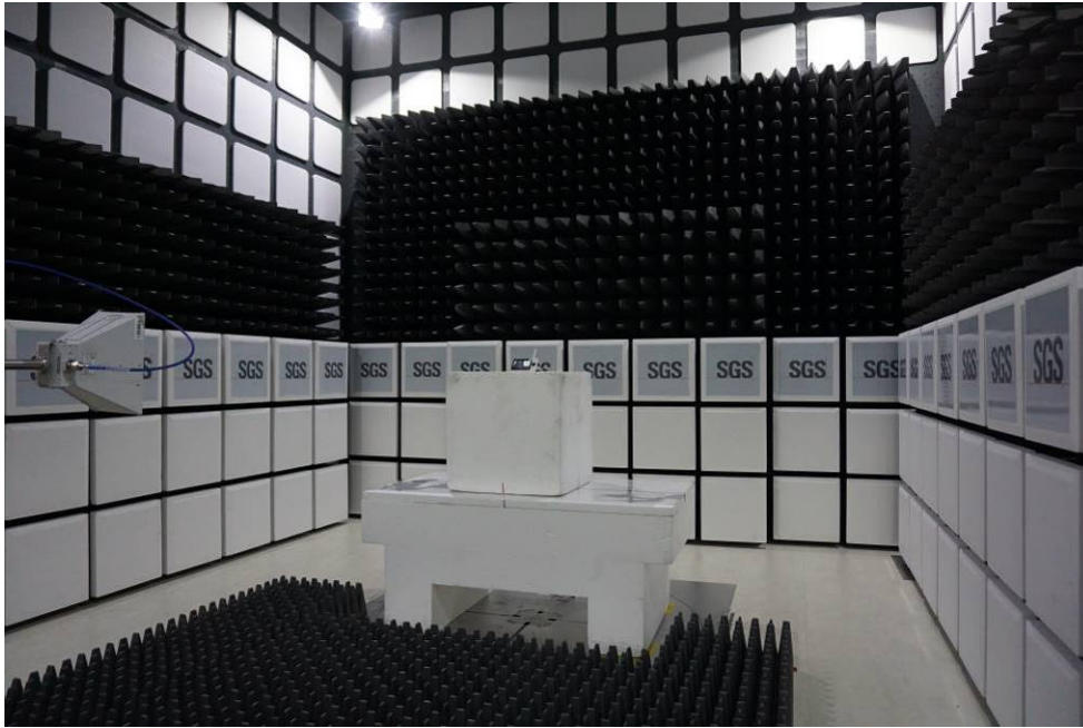
Radiated Emissions (Above 1GHz) Test Setup
