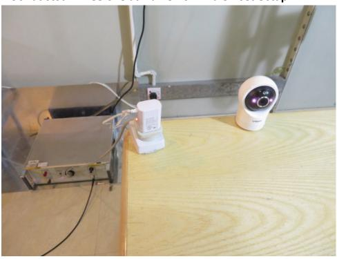
Radiated Emissions (30MHz-1GHz) Test Setup
