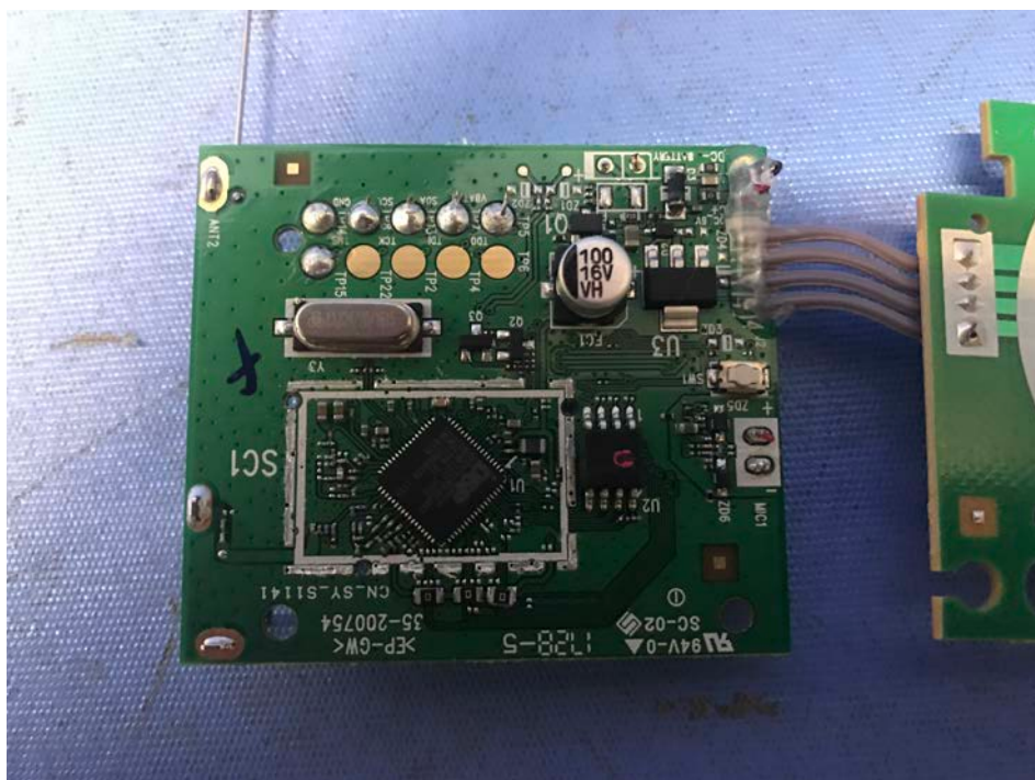
Left wire is antenna, right wire is as ground plane extension
