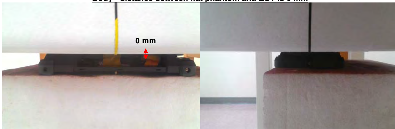
Fig.3 EUT Back side to flat phantom
