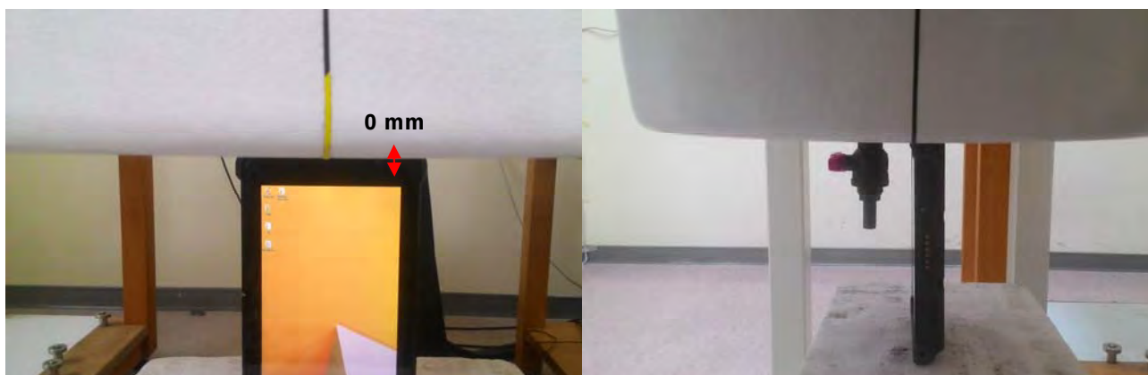
Fig.5 EUT Right side to flat phantom
