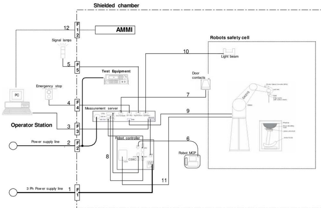
The DASY5 system for performing compliance tests consist of the following items:
