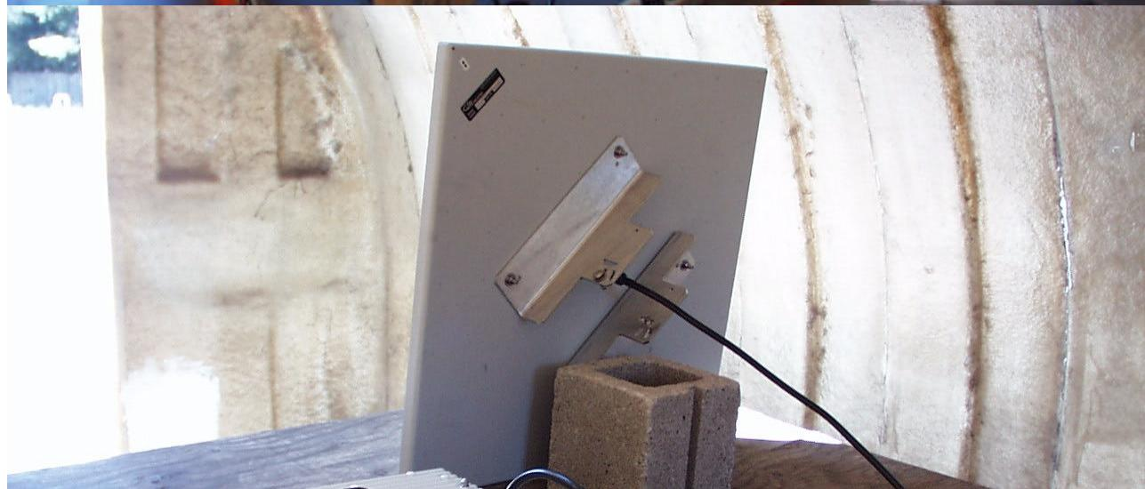
Antenna Used with Wireless Inc. 5.7 GHz Transmitter
