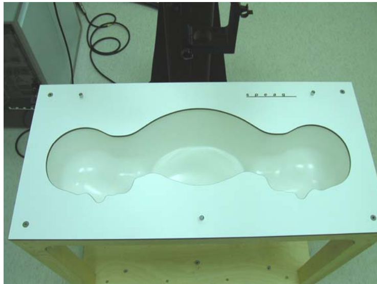
Fig. 5.3 Top View of Twin Phantom
