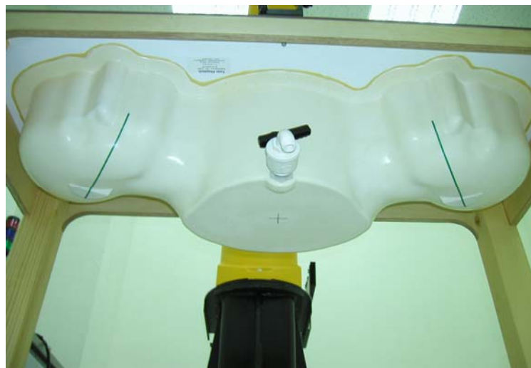
Fig. 5.4 Bottom View of Twin Phantom
