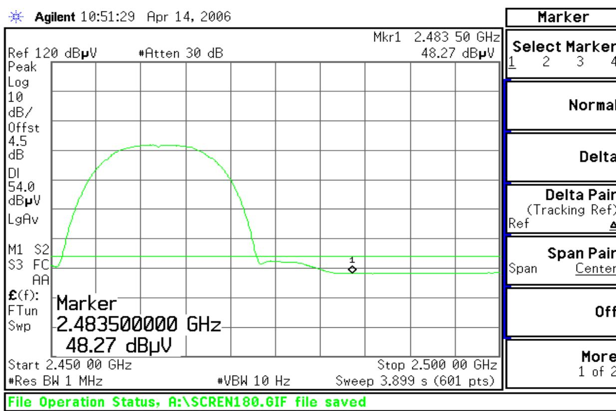
**Band Edges (802.11g / CH Low)****Detector mode: Peak****Polarity: Vertical**
