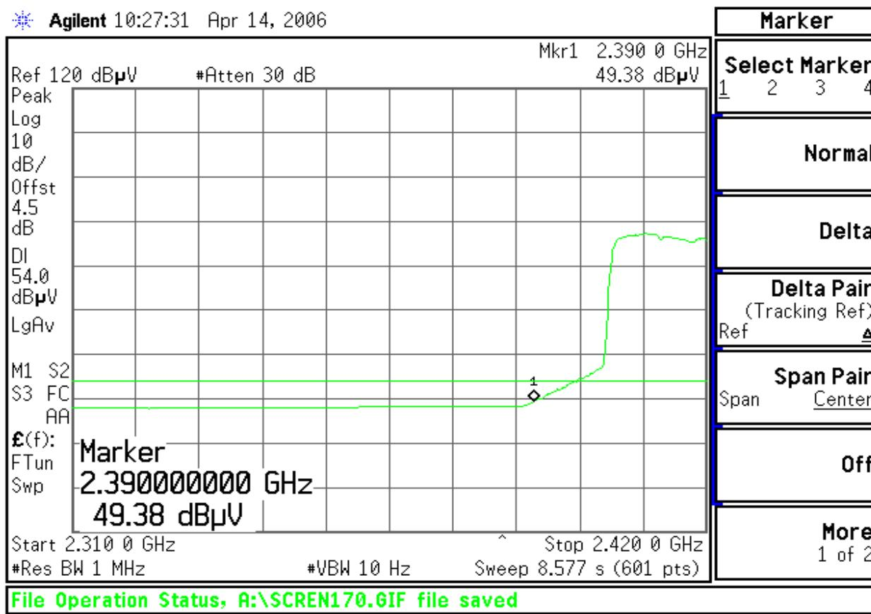
**Band Edges (802.11g / CH High)****Detector mode: Peak****Polarity: Vertical**
