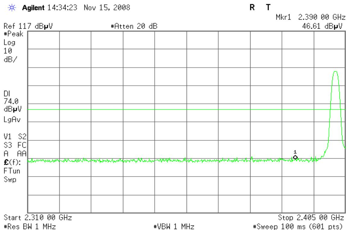
**Detector mode: Average****Polarity: Horizontal**
