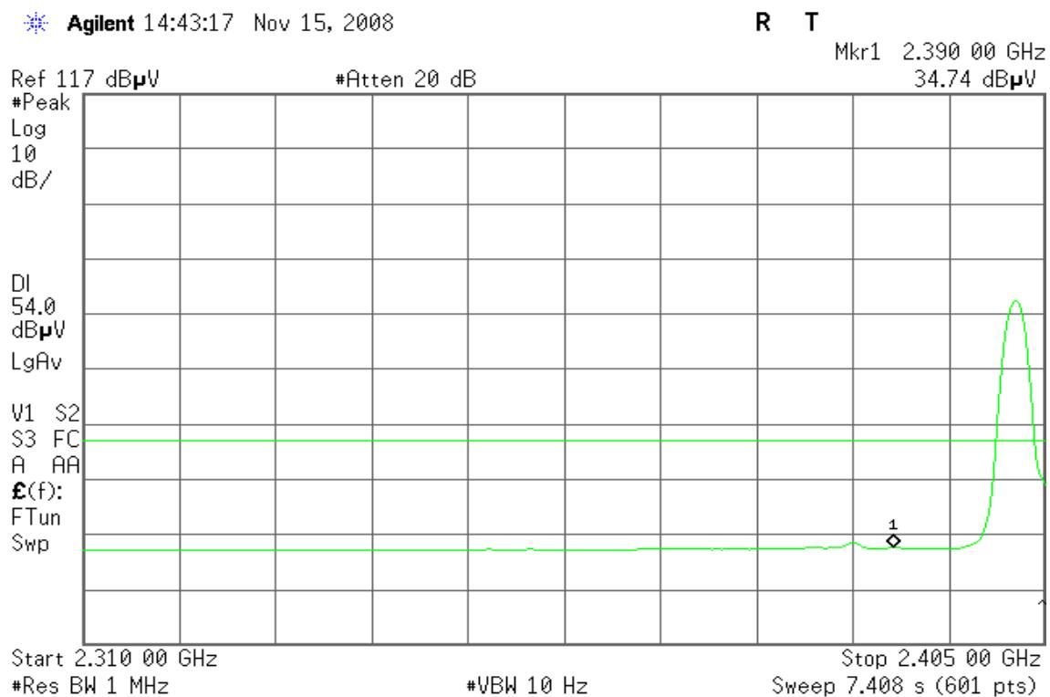
**Band Edges (CH High)****Detector mode: Peak****Polarity: Vertical**
