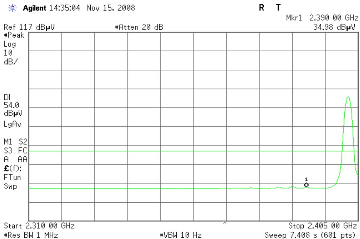
**Band Edges (CH High)****Detector mode: Peak****Polarity: Vertical**
