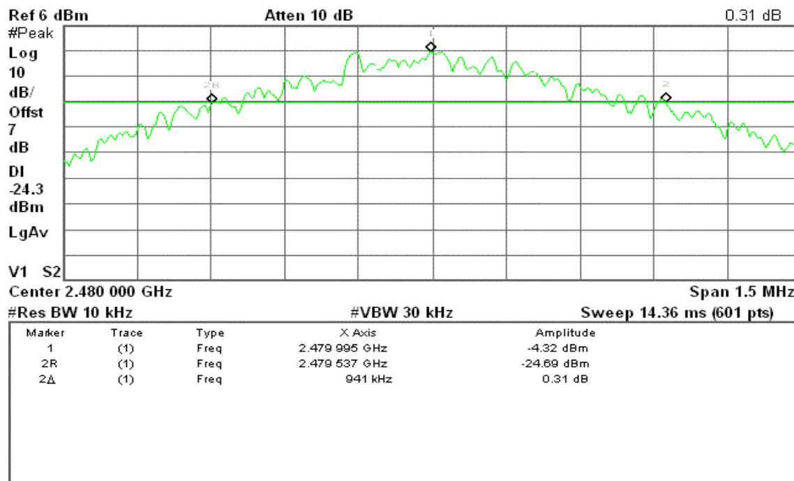
**For 8DPSK / DH5****20dB Bandwidth (CH Low)**
