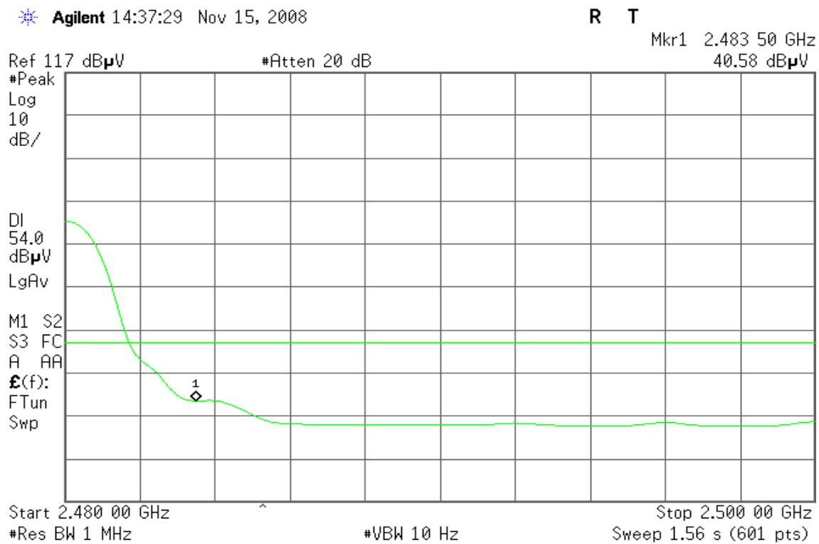
**For 8DPSK / DH5****Band Edges (CH Low)****Detector mode: Peak****Polarity: Vertical**
