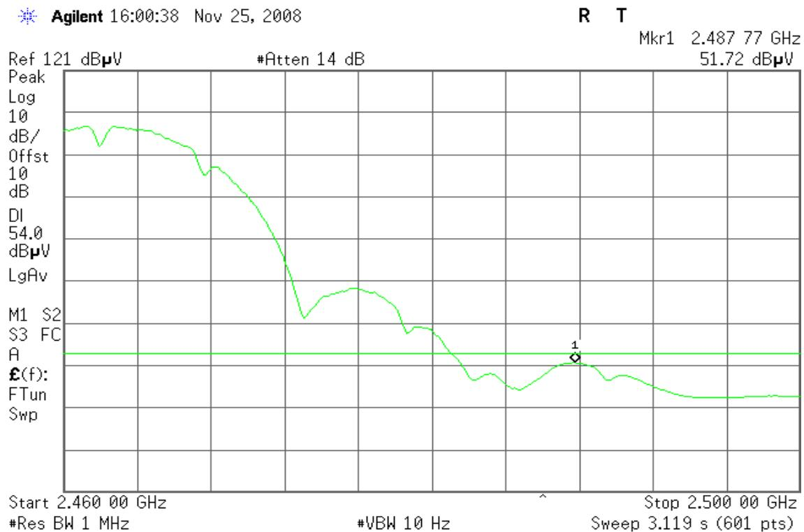
**Band Edges (IEEE 802.11g / CH Low)****Detector mode: Peak****Polarity: Vertical**
