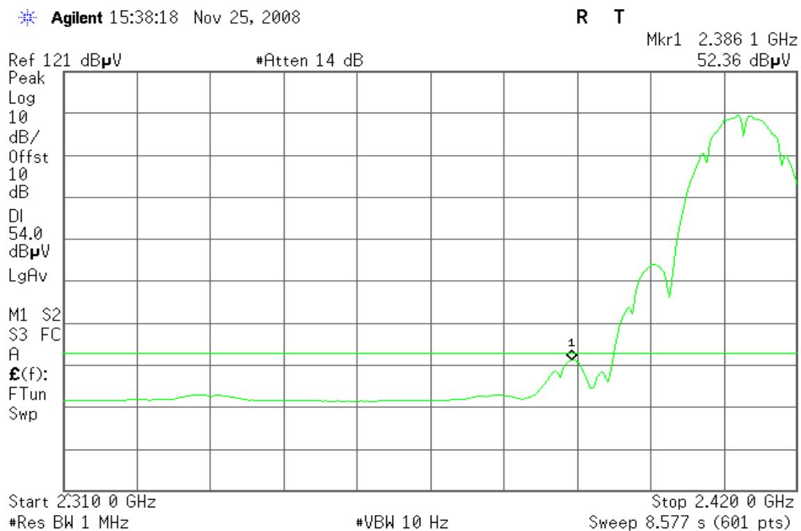
**Band Edges (IEEE 802.11b / CH High)****Detector mode: Peak****Polarity: Vertical**
