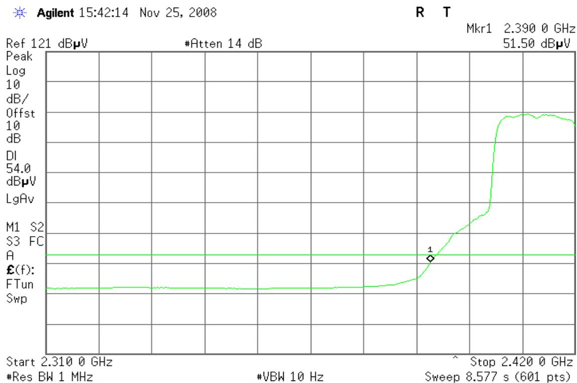
**Band Edges (IEEE 802.11g / CH High)****Detector mode: Peak****Polarity: Vertical**
