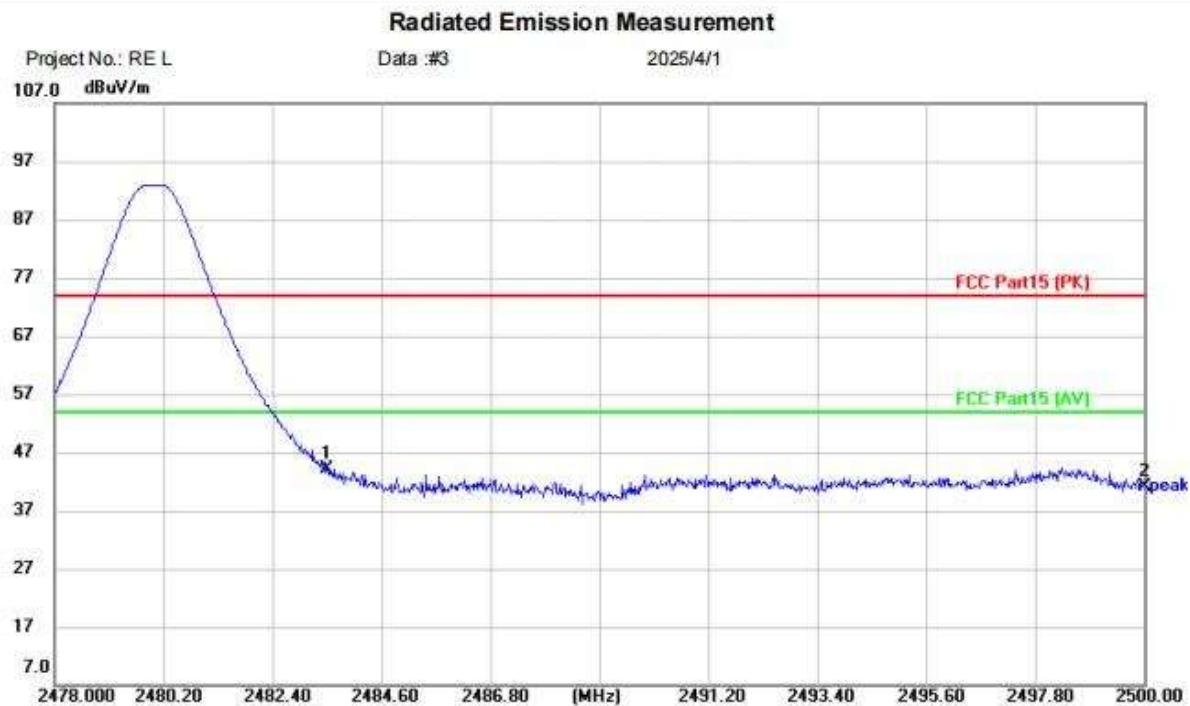
Site: Limit: FCC Part15 (PK) EUT: 4.1 Soundbar System M/N: SV410XW-0905 Mode: BT TX 2480 Note: Polarization: **Horizontal** Power: Temperature: (C) Humidity: %RH
