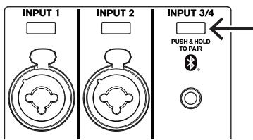
2. Navigate to your mobile device's Bluetooth® settings menu, find the EVERSE loudspeaker with the matching 4-digit ID and ensure you are paired to the loudspeaker. This will pair the mobile device to the EVERSE loudspeaker for audio streaming.
