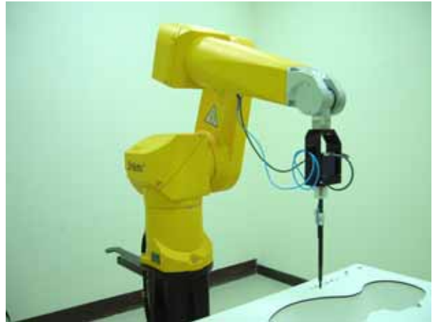
Fig. 5.2 Probe setup on robot
