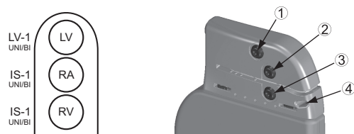
Figure 4. Lead connections and setscrew locations, RA: IS-1, RV: IS-1, LV: IS-1
