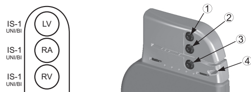
Figure 4. Lead connections and setscrew locations, RA: IS-1, RV: IS-1, LV: IS-1
