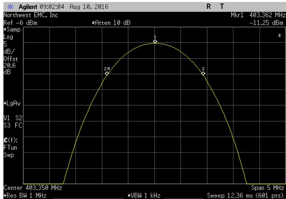
Extreme Voltage +15% (138VAC/60Hz), Mid Channel, 403.35 MHz
