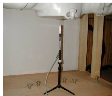
Figure 12-2 System Verification Setup Photo
