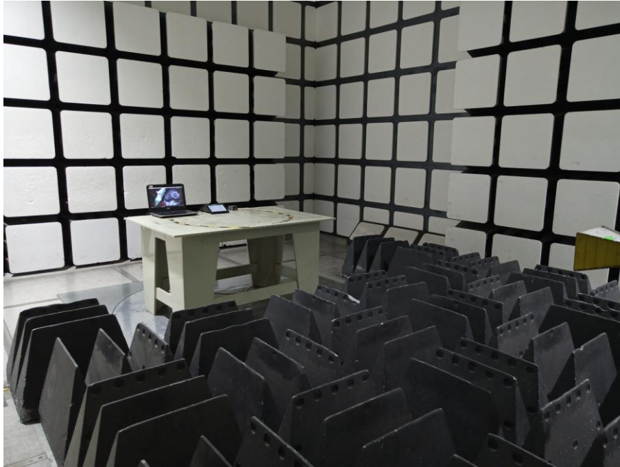
Radiated Emissions – Front View (Above 1 GHz)
