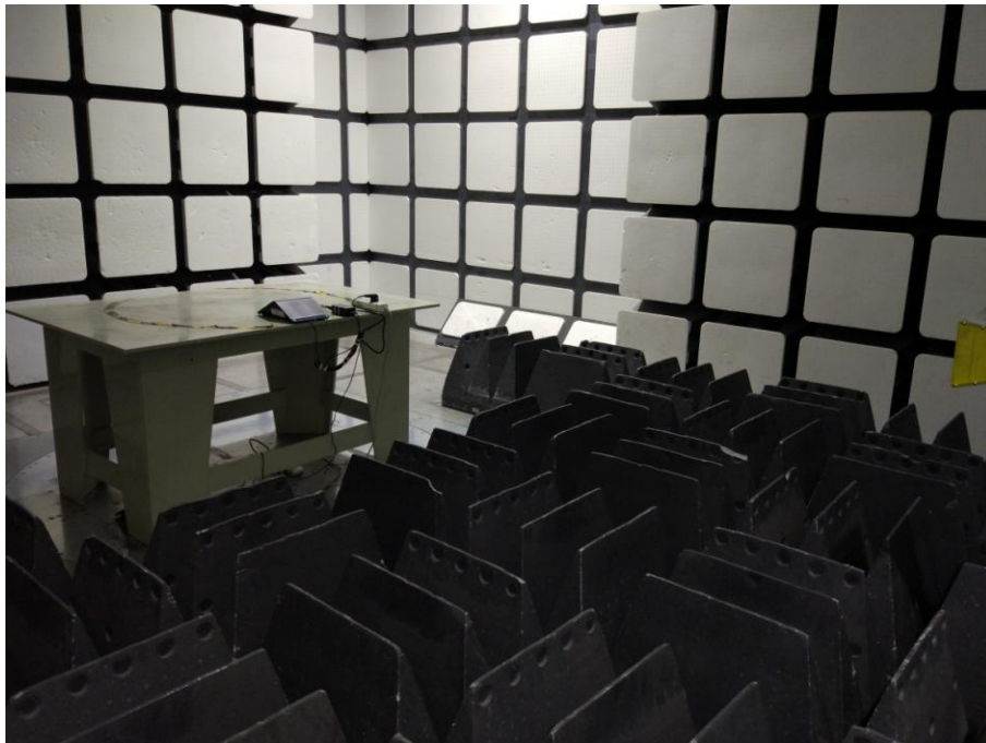
Radiated Emissions – Rear View (Above 1 GHz)
