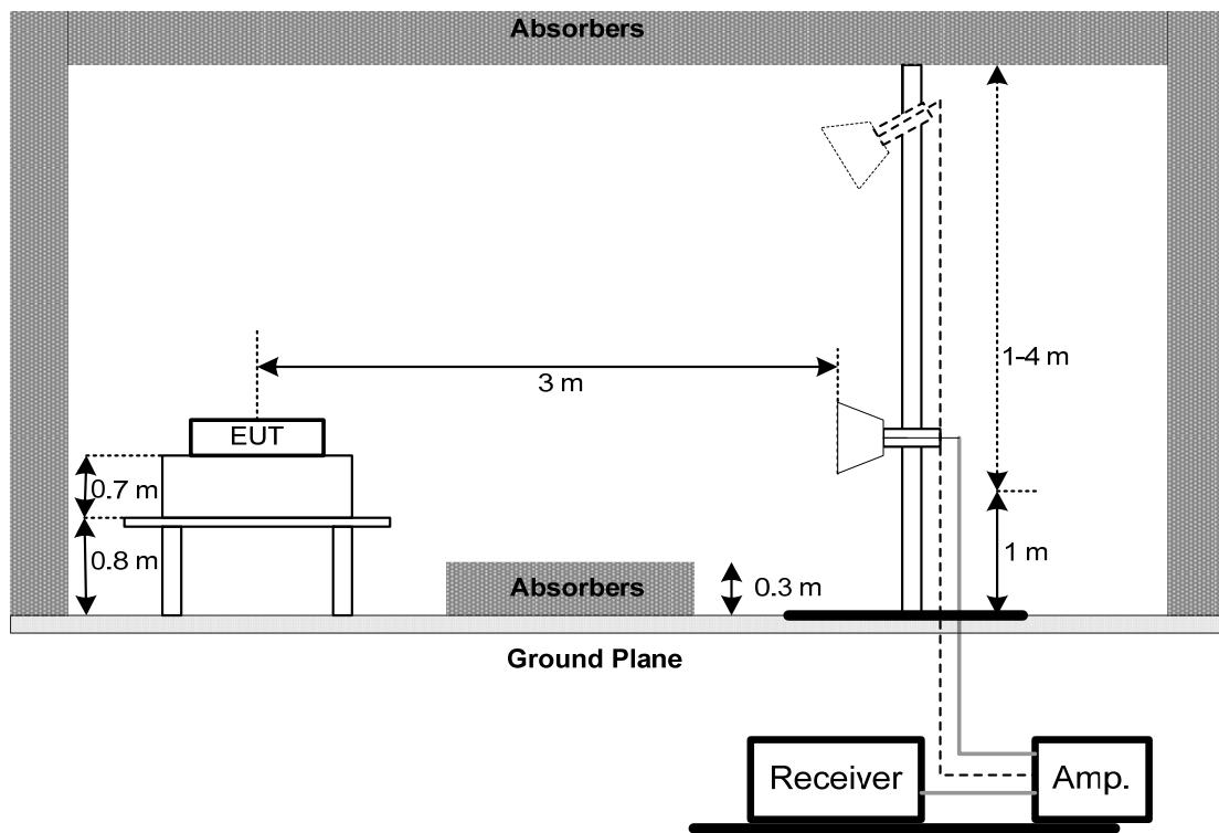
(C) For radiated emissions below 30MHz
