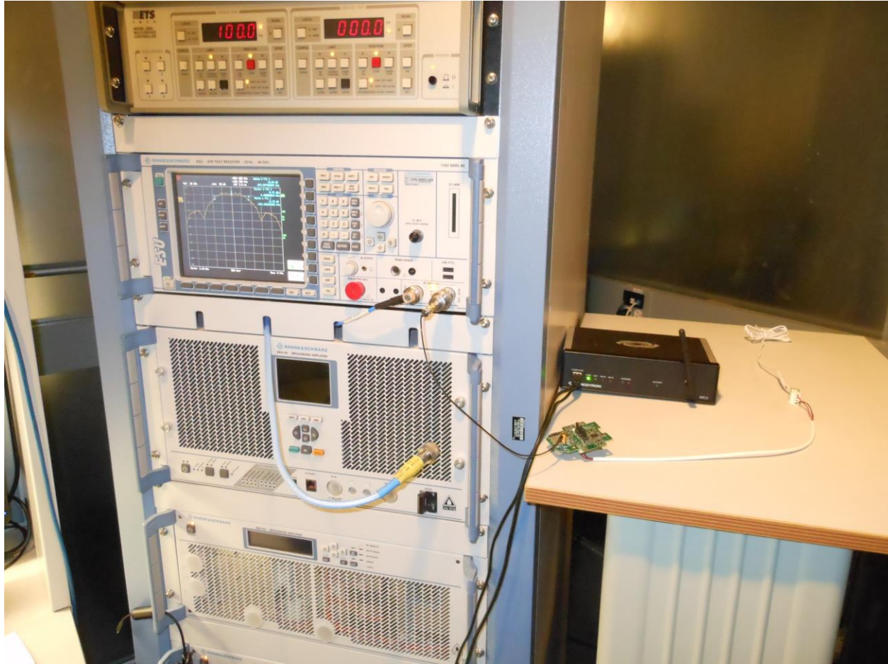
Antenna port conducted measurement on radio board
