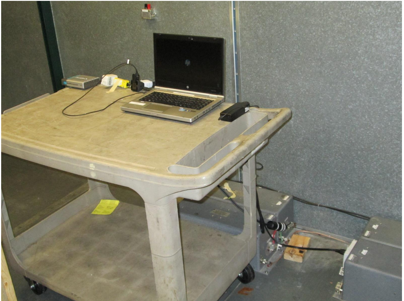
Figure 3 Test Setup for Conducted Emissions
