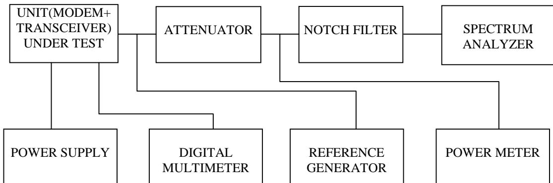
NAME OF TEST: Transmitter Spurious and Harmonic Outputs
