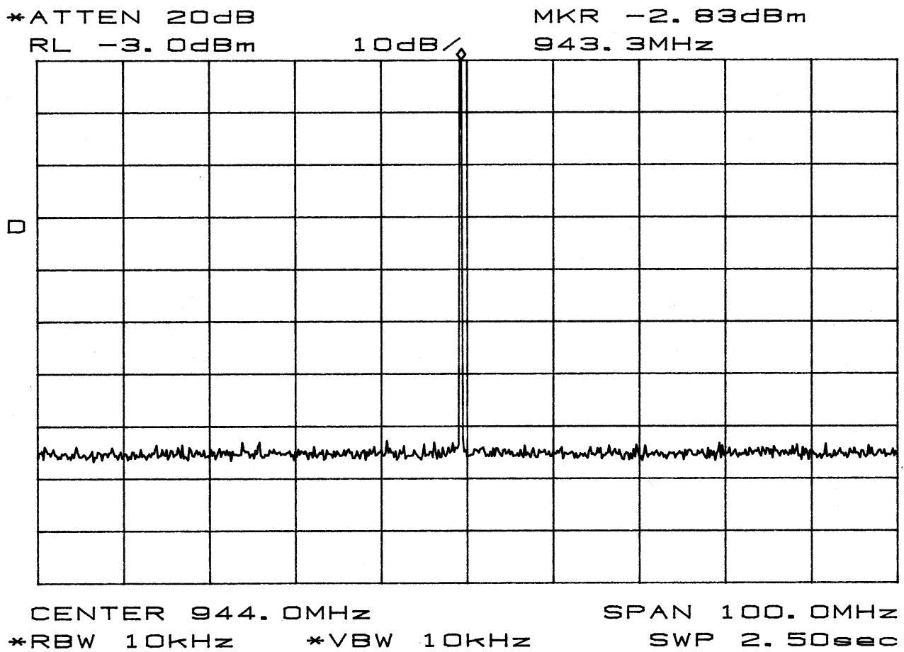
NAME OF TEST: Transmitter Occupied Bandwidth
