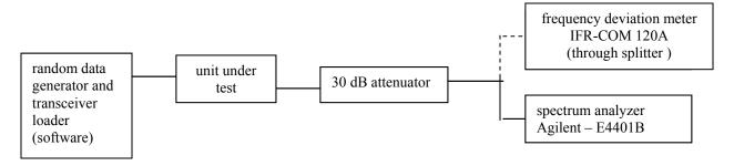
NAME OF TEST: Transmitter Occupied Bandwidth
