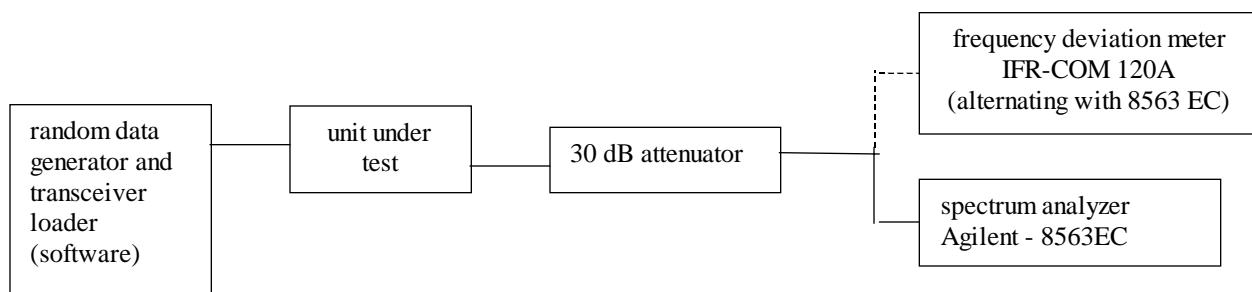
NAME OF TEST: Transmitter Occupied Bandwidth
