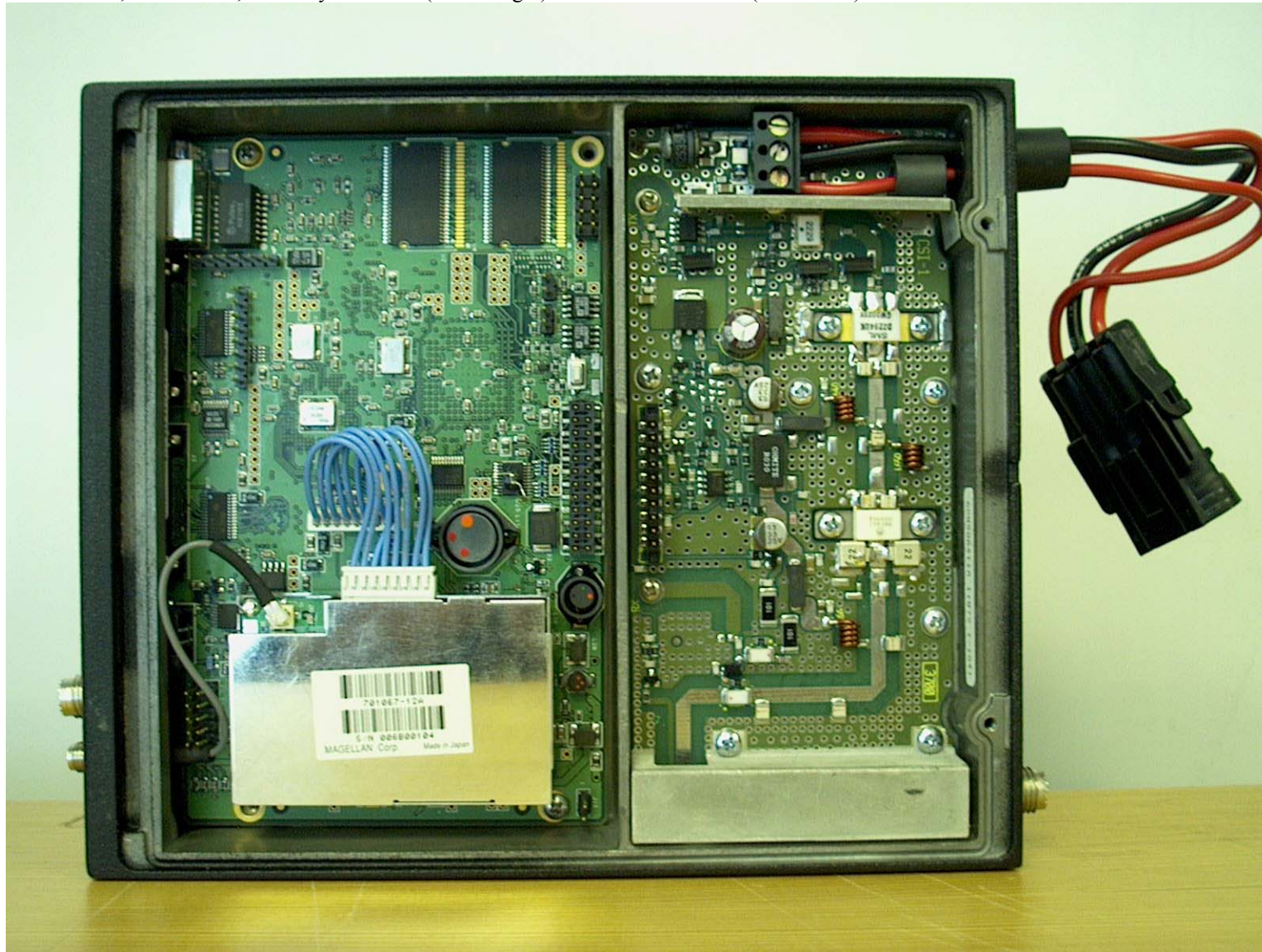
Bottom view, lid removed, assembly PA board (toward right) and G3 modem board (toward left)
