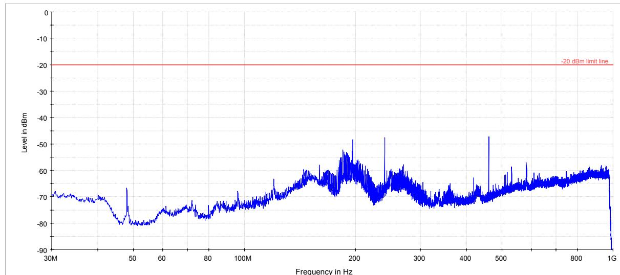
Radiated spurious emissions on P4 with SDR-001-T-438
