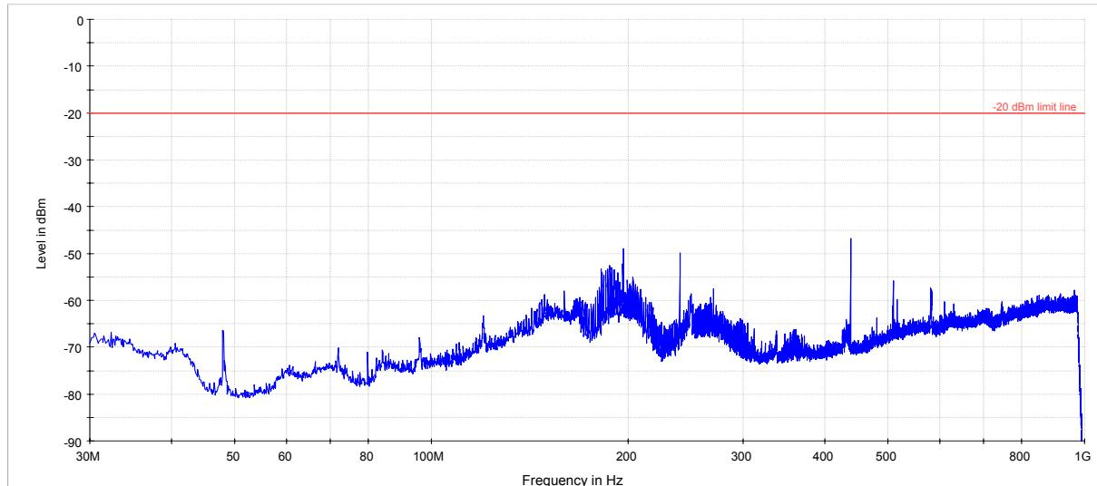
Radiated spurious emissions on P4 with SDR-001-T-438
