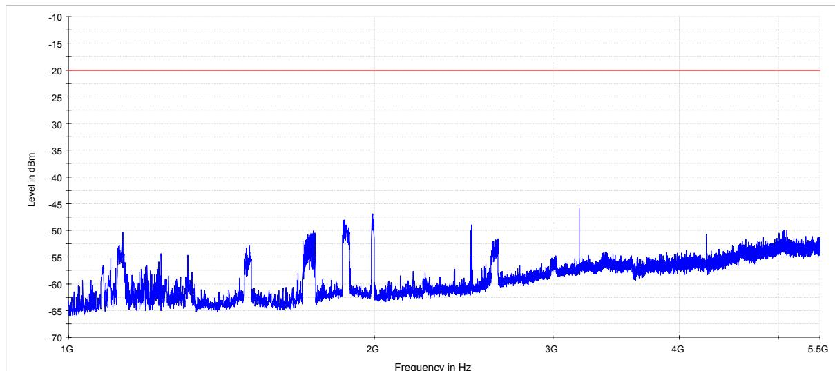
Radiated spurious emissions on P4 with SDR-001-T-438
