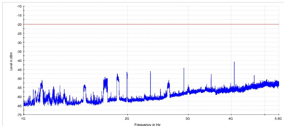
Radiated spurious emissions on P4 with SDR-001-T-438
