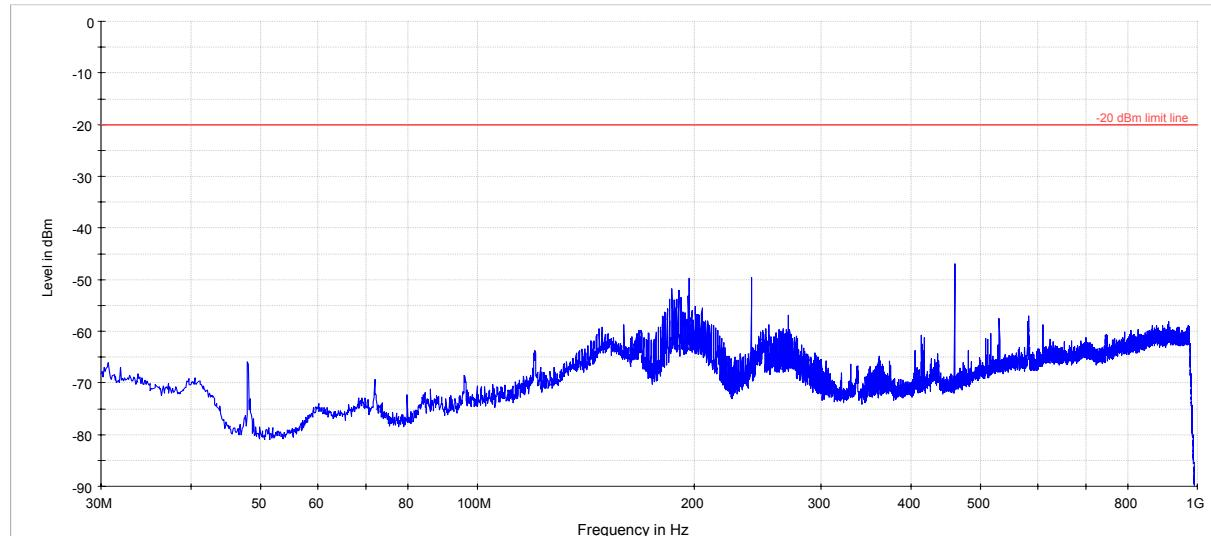
Radiated spurious emissions on P4 with SDR-001-T-438
