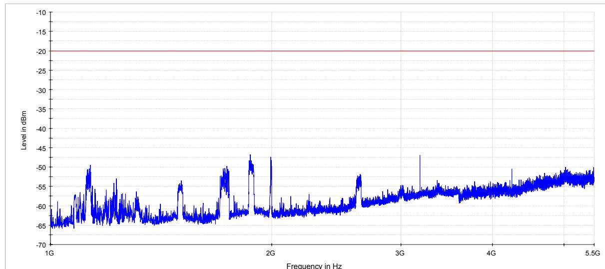
Radiated spurious emissions on P4 with SDR-001-T-438
