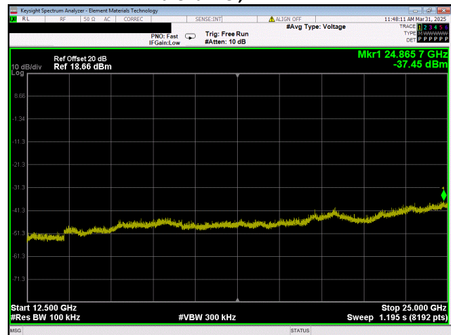
BLE/GFSK 1 Mbps Mid Channel, 2442 MHz
