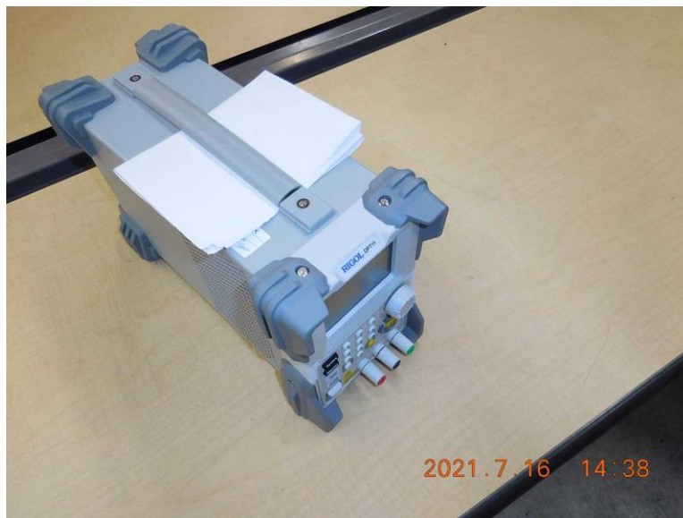
DC Power Supply
