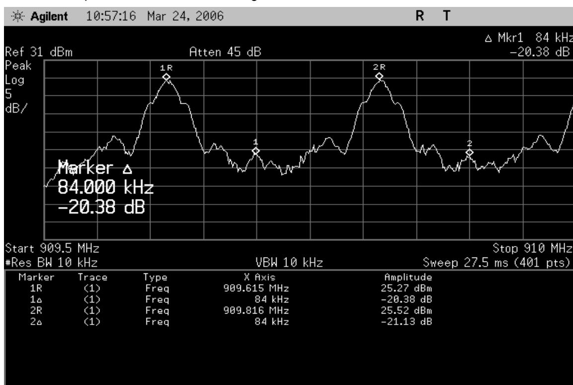
Plot # 2 carrier separation is 203 kHz. This is greater than the max 20 dB BW of 131.3 kHz.
