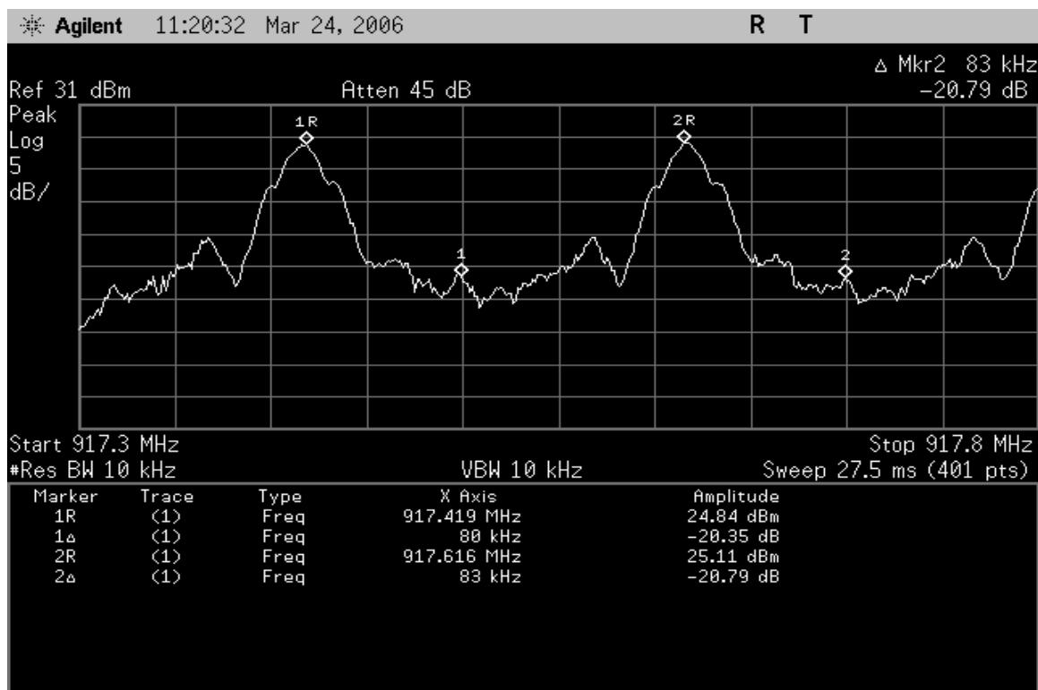
Plot # 4 carrier separation is 197 kHz. This is greater than the max 20 dB BW of 131.3 kHz.
