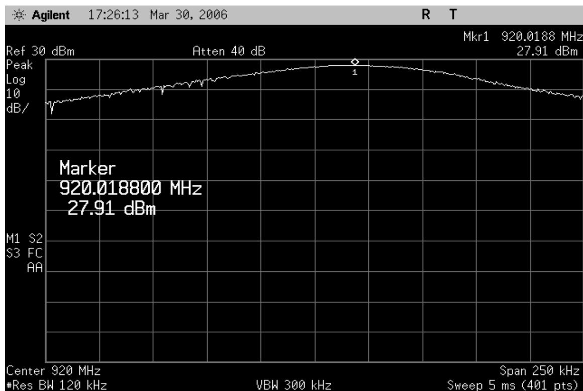
Following readings @ 95 V<sub>rms</sub> input.
