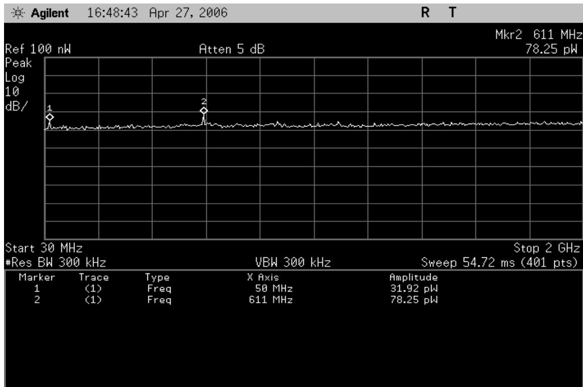
The receiver was set to RX on frequencies 910,911,912,915,916,918,919,920. This band as well as the 2<sup>nd</sup> and 3<sup>rd</sup> of this band were checked.
