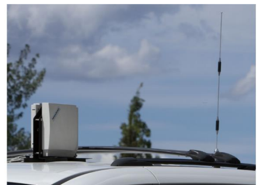
Figure 5: Vehicle with installed GPS Antenna, Mobile Whip Antenna, and Side Looker Receive Antenna array
