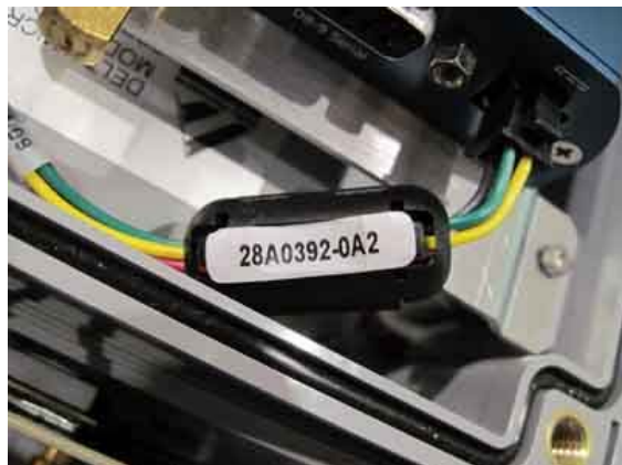
FERRITE ON CELL MODEM POWER CABLE
