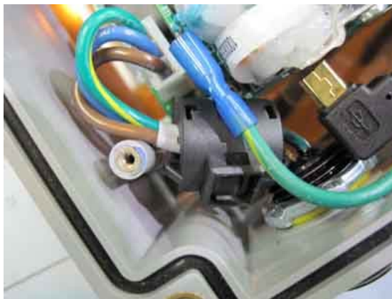
FERRITE ON INPUT POWER CABLE
