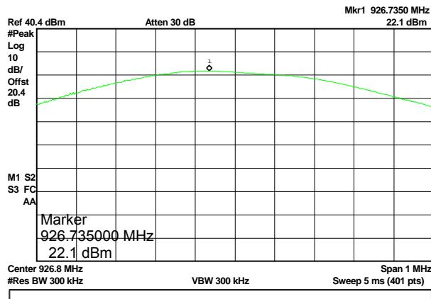
Note 1: The path loss for the cavity filter used in the transmitter path is specified at 5.0 dB max (924MHz - 926MHz) and 12dB min at 928 MHz. Therefore, at 926.8 MHz the output power could be 10dB lower than mid band power at 915 MHz.
